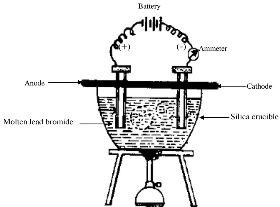
1. Why is a silica crucible used for the electrolysis of PbBr<sub>2</sub>? [1]
