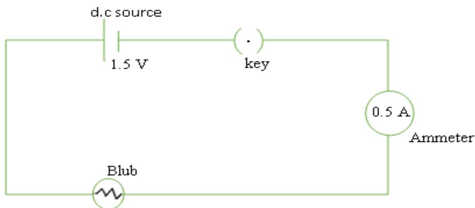
Calculate the resistance offered by the bulb.
