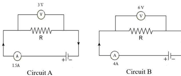
i. Calculate the resistance for circuits A and B. [1]
